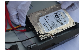
Figure3-2 Insert hard disk data cable and power cable
